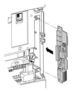
• First remove the empty option card support (if present), as indicated on the previous page, so you can access the slot for the encoder feedback card.
