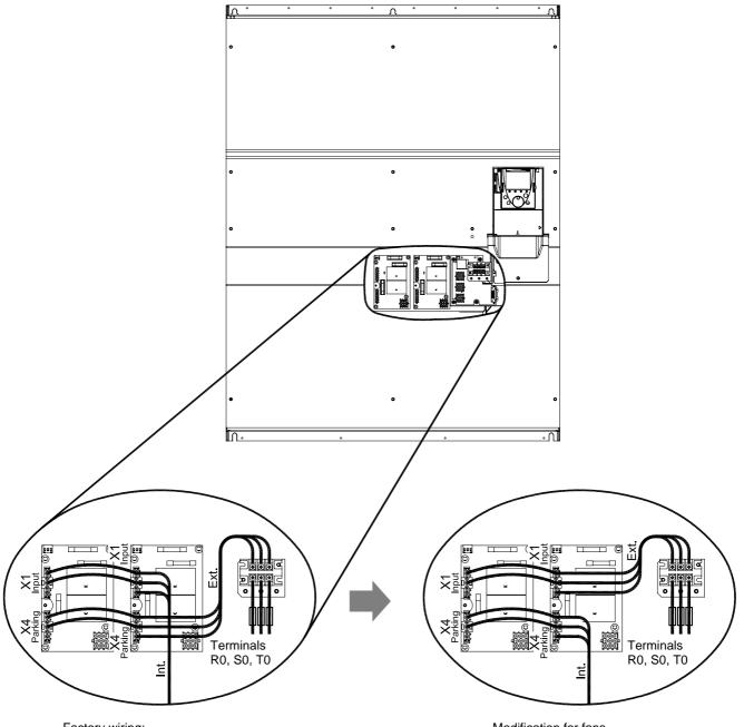
Factory wiring: fans powered internally by R/L1, S/L2, T/L3
