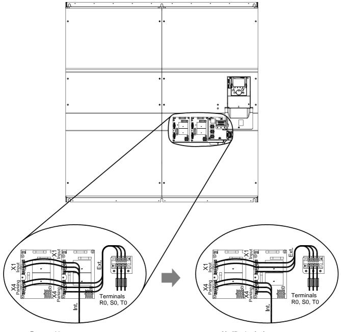
Factory wiring: fans powered internally by R/L1, S/L2, T/L3
