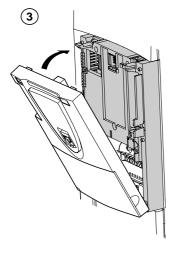
(3) Replace the control front panel on the option card (same procedure as for installing the option card, see (1) and (2))
