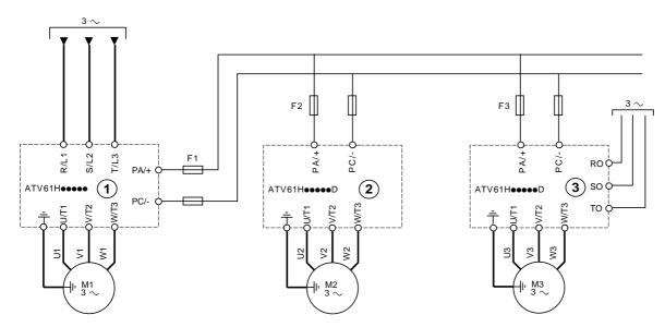
Drives (2) and (3) powered only by their DC bus do not necessarily have a DC choke (catalog number ATV61••••D).
