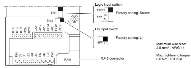
**Note**: The ATV61 is supplied with a link between the PWR and +24 terminals.
