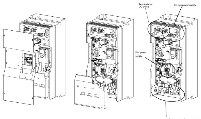
Power section line supply Output to the motor Connections to ground Output to braking resistor (up to ATV61HC16N4 rating only)
