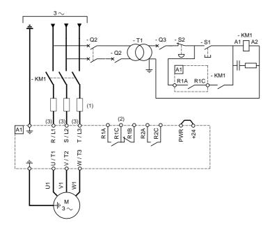
**Diagram with switch disconnect**
