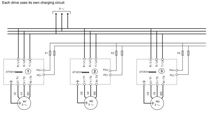
Drives (1), (2) and (3) must not be more than one size apart when they are connected in this way.
